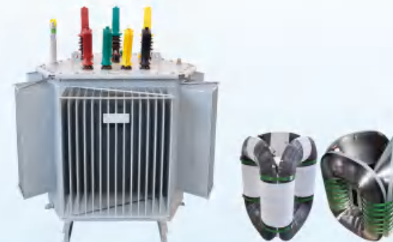
10~35kV Series Oil-Immersed Tridimensional Toroidal Core Distribution Transformer
